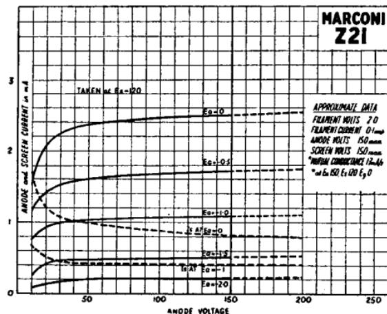
Marconi Z21 is a screened pentode for use where a variable mu characteristic is not required. In particular it makes a sensitive grid detector
