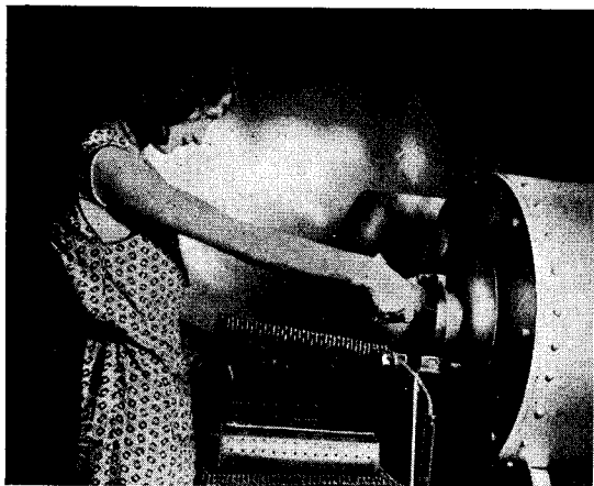
One of the 20 ft. hydrogen-filled electric furnaces in which metal valve parts are heated to 1000° C. in order to remove all occluded gas and foreign matter.
