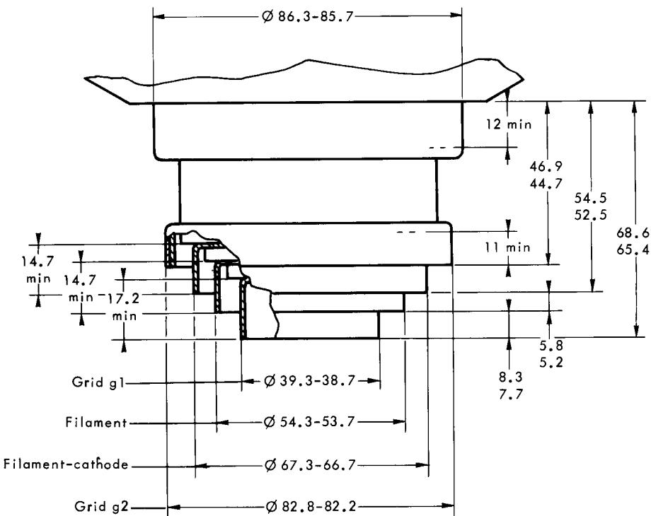
DETAIL OF COOLING APERTURE ON G1, FK, F CONNECTIONS
