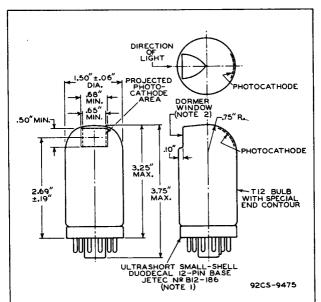
NOTE 1: ¢ OF BULB WILL NOT DEVIATE MORE THAN 2° IN ANY DIRECTION FROM THE PERPENDICULAR ERECTED AT THE CENTER OF BOTTOM OF THE BASE.
