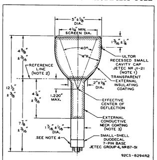
**NOTE 1:** THE PLANE THROUGH THE TUBE AXIS AND VACANT PIN POSITION 3 MAY VARY FROM THE PLANE THROUGH THE TUBE AXIS AND ULTOR TERMINAL BY AN ANGULAR TOLERANCE (MEASURED ABOUT THE TUBE AXIS) OF  $\pm$  10°. ULTOR TERMINAL IS ON SAME SIDE AS VACANT PIN POSITION 3.
