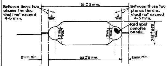
The leads shall be flexible 26 S.W.G. tinned wire not less than 3" in length. There shall not be excess solder on the connection of the lead to the tungsten lead-out.
