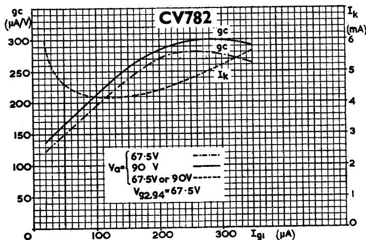
Conversion Conductance and Cathode Current plotted against Oscillator Grid Current
