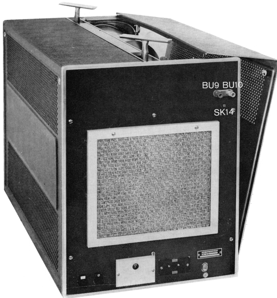
Fig. 4b. Rear view with Z-modulation input terminals and switch
