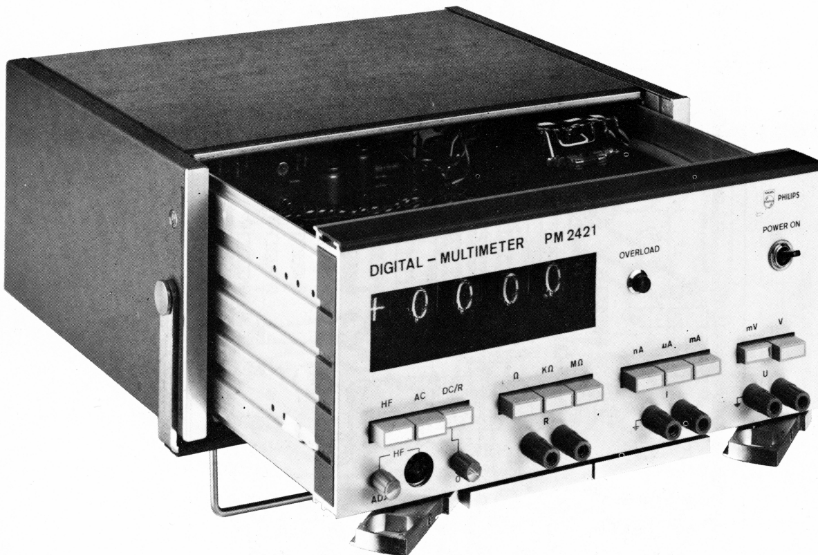
Fig. 42. Pulling the instrument chassis out of the cabinet
